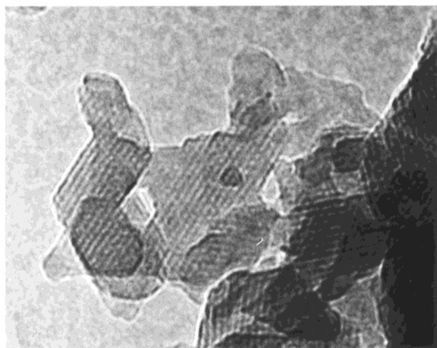
Figure 3. Further magnified view of the central-left region in Figure 2A to show hexagons and a trigon on top of a faceted and columnar hexagonal colony of silicate MCM-41. The tubular interspacing is ca. 5 nm.
